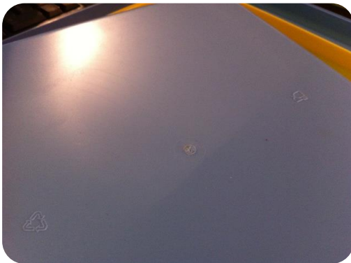
Poor injection quality
