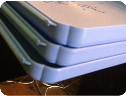
Sides without any slope, resulting unfixing problem
